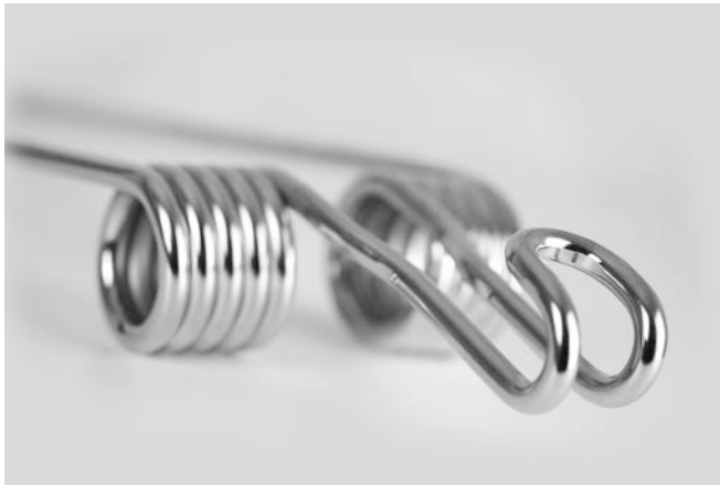
Fig. 1 Typical wire coil part (tedder fork), produced ready-for-use on a BM 90 single-head wire bending machine.
