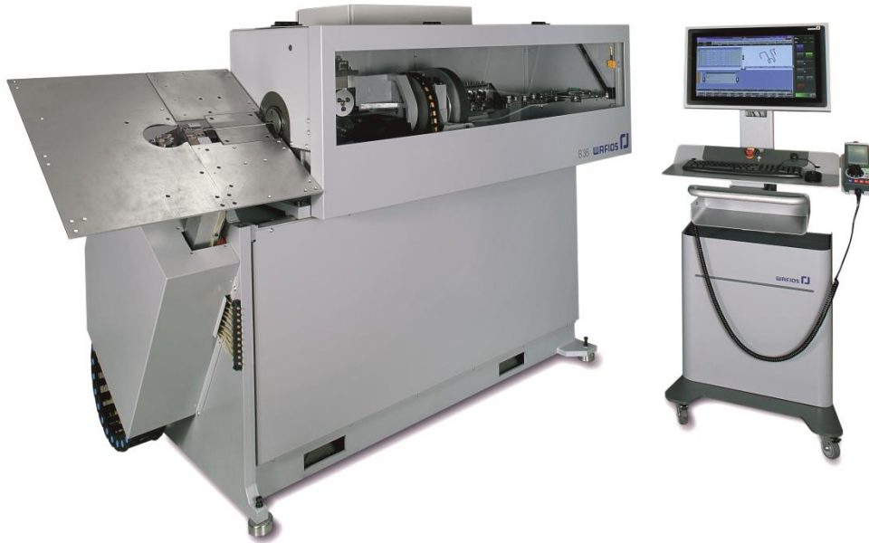
Fig. 3 The WAFIOS B 36 Performance single-head wire bending machine is the latest model in the B series. First machine in this series with the WPS 3.2 EasyWay programming system.
